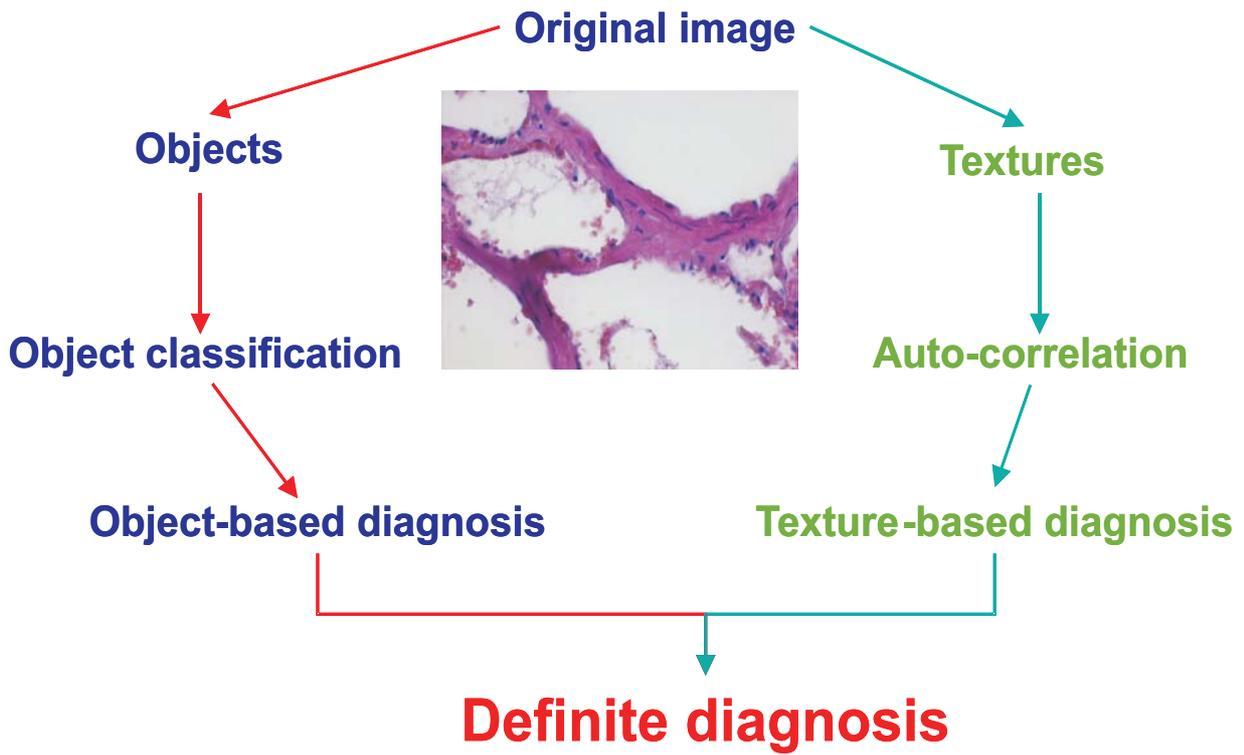
Figure 3 – Scheme of object and texture related feature extraction to computing tissue-based diagnoses
