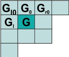
Using  $S = E( [a_{10}G_{x-1,y-1} + a_0G_{xy-1} + a_{x0}G_{x+1,y-1} + a_1G_{x-1,y} + R_{x,y} - G_{x,y}]^2 ) \rightarrow \text{minimum}$
