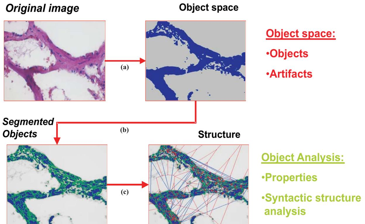
Figure 4 – The algorithm to analyzing object associated image information includes: (a) a separation of the image into object space and background, (b) object segmentation and identification within the object space, and (c) syntactic structure analysis to identifying spatial relationships between identified objects
